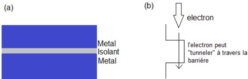
Fig. 1 (a) Schematic of a tunnel junction. (b) Electron tunneling through an energy barrier.
